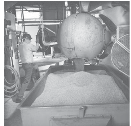
All Briess caramel malts are roasted. We operate both drum and traditional ball roasters (pictured above).
