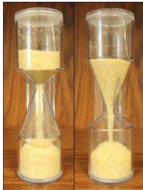
Not all silos are shaped alike as these acrylic models demonstrate. Talk to your silo manufacturer how this affects the flow of the malt.
